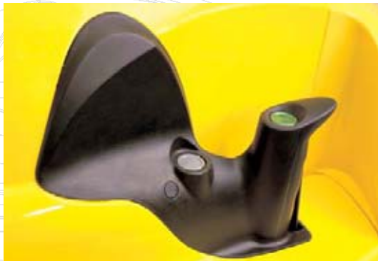
Featuring piezo technology, the right Controlgrip with its Powergrip is used for acceleration.
